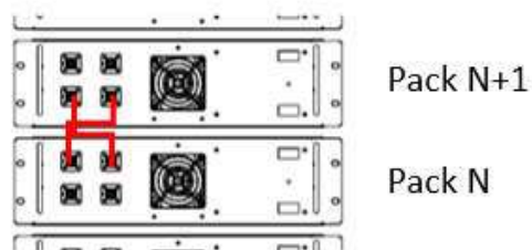
Wrong connection mode 3
